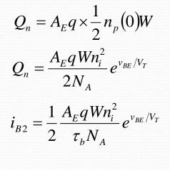
$$i_B = I_S \left( \frac{D_p}{D_n} \frac{N_A}{N_D} \frac{W}{L_p} + \frac{1}{2} \frac{W^2}{D_n \tau_b} \right) e^{v_{BE}/V_T}$$
